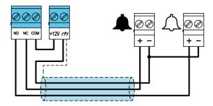
In this connection mode, it is possible to activate both the external sounder and any internal sounder at the same time through the voltage-free "COM-NC-NO" relay of the control panel. Switching the relay disconnects the "+" terminal of the external sounder and at the same time connects the "+" of the internal sounder.
