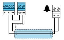
This standard wiring method activates the alarm signal by means of a positive-power-removed signal.
