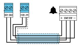
This connection mode allows greater flexibility for activation/deactivation of the sounder.
